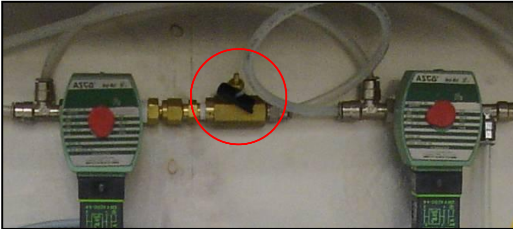
Figure 20. Adjust Nitrogen needle valve (in compartment beneath oven).
