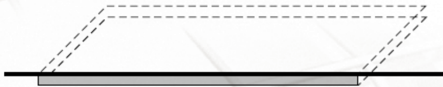
Recess mounted, insulating cement and 1/4" steel plate
